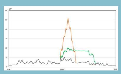
The orange line represents the situation if four of them would have an EV, and all EVs would charge 20 kWh, without any incentive at all. The first starts charging at 17:30, the others at 18:00, 18:30 and 19:00 respectively. The green one is exactly the same situation but now with an incentive for each customer to keep the individual total load (kW) low. Now each customer just takes more time to charge 20 kWh into the EV, resulting in a reduction of the total simultaneous load on the grid.
