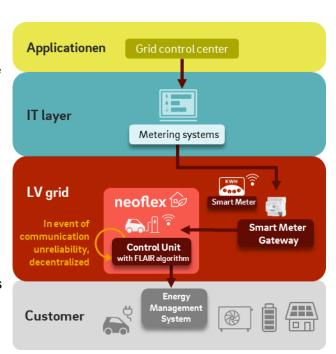
The neoflex algorithm is designed to run in a control unit or, in the future, in smart meter gateways. While the system's functioning is **independent of communication reliability**, its integration with the smart meter gateway remains possible. In Germany, this represents an additional fallback solution for centralised control of flexible loads. At the same time, neoflex could be implemented internationally as a new stand-alone solution.
