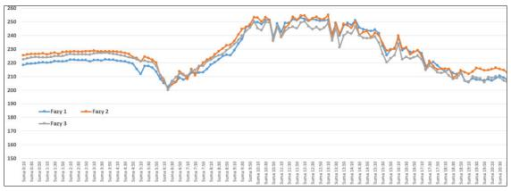
Phase voltages on the customer side after the installation of a Phase Balancer. The voltage fluctuates depending on the time of day, but the difference in deviation between phases is much lower compared to before the installation of the device.
