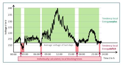
The neoflex algorithm calculates the local and individual blocking times per household based on voltage measurement data.
