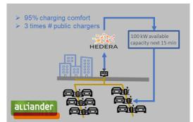
capacity is significantly smaller than the sum of the technical charging capacity of each charging point so more public chargers can be connected to the LV grid without overload risks. Additionally, to the firm group capacity and according to the current grid status, Alliander can release **near real-time additional non-firm capacity** which the CPO is allowed to use for free.
