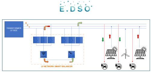
Working principle. In this example, the LV Network Smart Balancer allows energy transfer from a high-generation phase (S). to a high-consumption phase (R).
