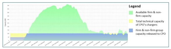
Example of HEDERA capacity allocation to the CPO based on available grid capacity. The extra non-firm capacity released at night (in green) and the dynamic limitation of allocated capacity during day and evening hours are clearly visible.
