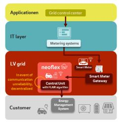
The neoflex algorithm is designed to run in a control unit or, in the future, in smart meter gateways.
