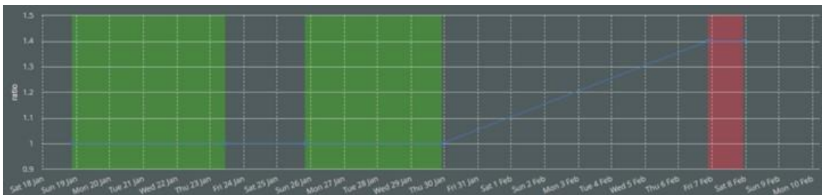
Image 3: Tampering ratio evolution. The meter tampering ratio is defined as \text{ratio} = \text{consumed energy} / \text{registered energy} . In the chart, green means \text{ratio}=1 (not tampered) and red means \text{ratio}>1 (tampered). The grey zones indicate that the algorithm is working on a new result.
