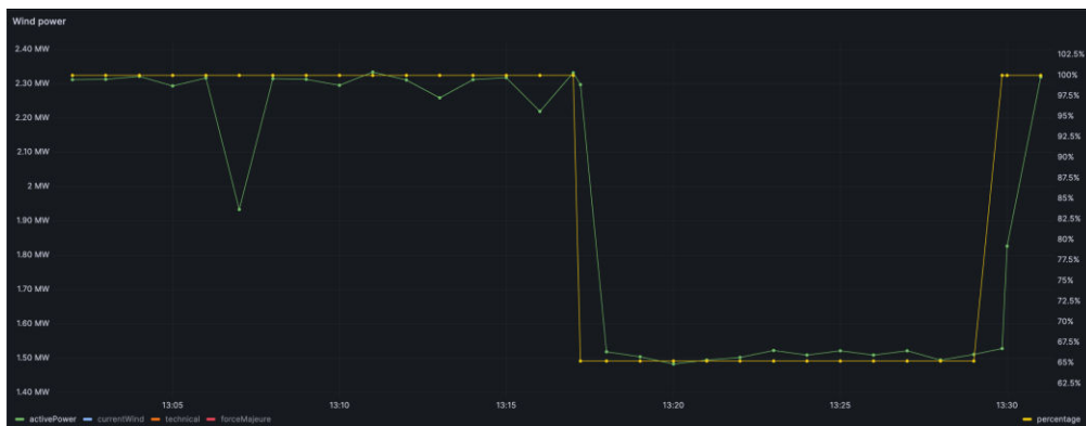
Example of a real-life emergency curtailment. The grid user reduced its infeed in just 1 minute (see communicated setpoint in yellow and real infeed measurement in green).
